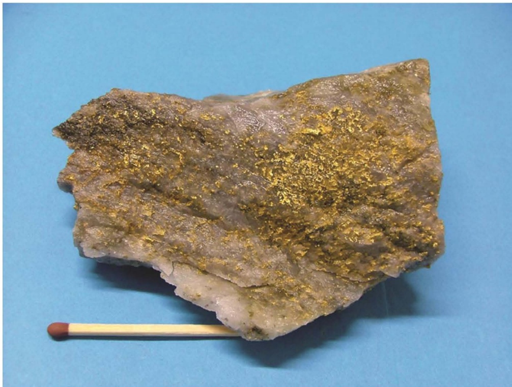
Fig. 3. Gold flakes in quartz with greyish to brownish parts containing fine grained gold (Foto: H. Buus Madsen).
