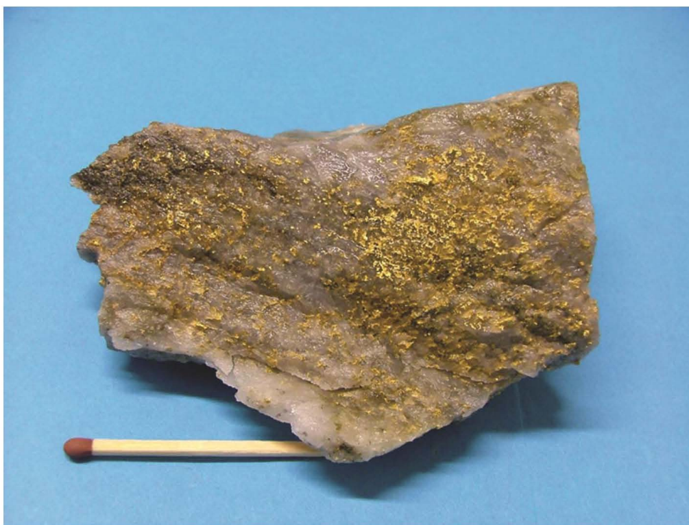
Fig. 3. Gold flakes in quartz with greyish to brownish parts containing fine grained gold (Foto: H. Buus Madsen).
